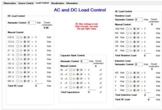
Load control user interface – Micro controllers
